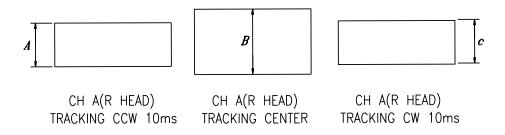
Fig. 5-11 X-POSITION ADJUSTMENT
